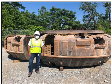
Photo: Courtesy of Indianapolis Dept. Of Public Works Tunnel boring machine in the Belmont North Relief Interceptor, added to the plan.
